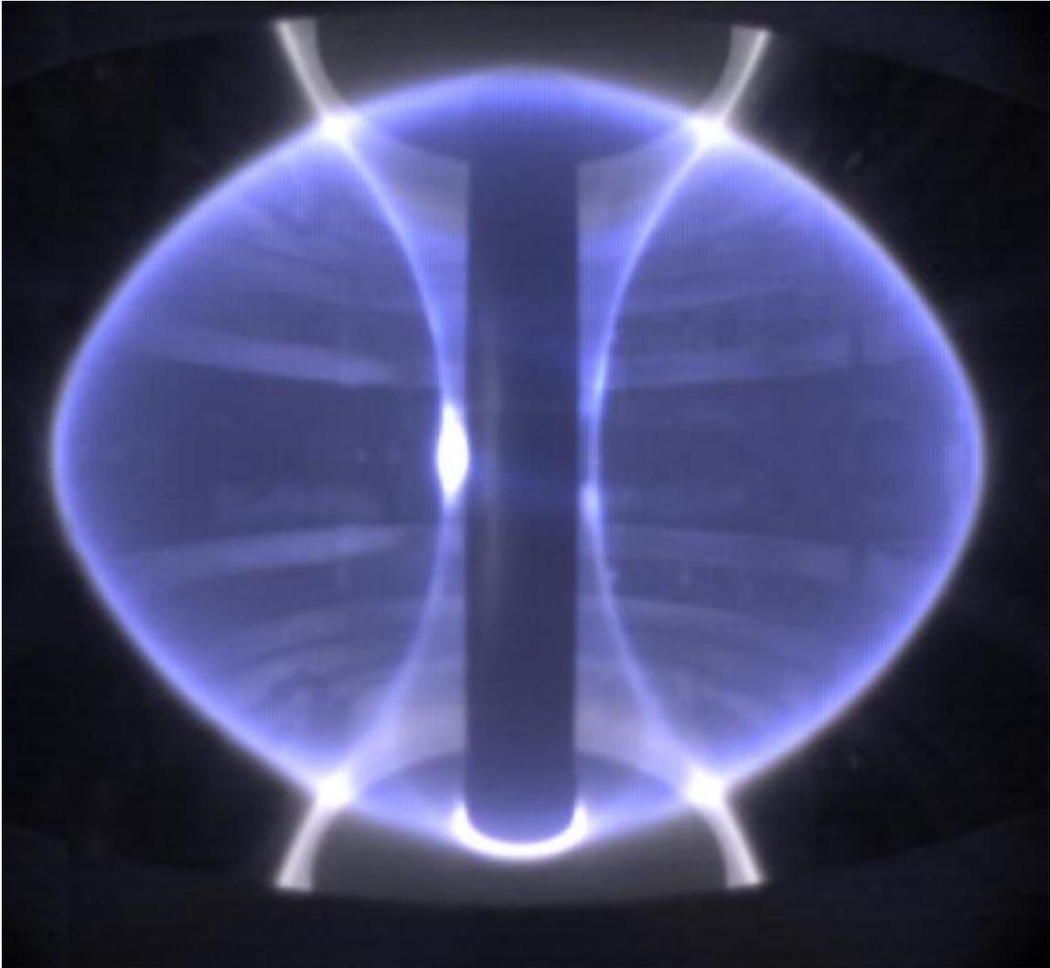
*A Plasma in MAST (Mega Amp Spherical Tokamak)*
