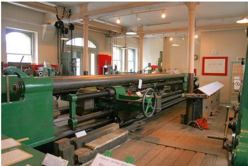
Key to this was his 'universal testing machine'. Built in Leeds, the machine was installed initially in premises in The Grove, off Southwark Street, London SE1, opening on 1st January 1866. Rapidly earning a worldwide reputation meant expansion with staff and equipment moving to a specially designed building at 99 Southwark Street where business began on 1st January 1874.
